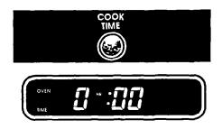
Turn the Time/Temp Set Knob clockwise until the desired baking/roasting time shows in the large display.
